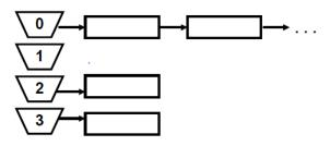
3) When the resource is search, its hash is obtained using hashing algorithm and then the latch is obtained to find the corresponding hash bucket and then the resource is search on the list in hash bucket. If the resource is found, Lock structure is obtained and the request is placed on owner, waiter and convert list as per the specified level of lock requested
